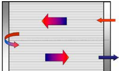
Figure 2: Typical 2-Pass Construction
